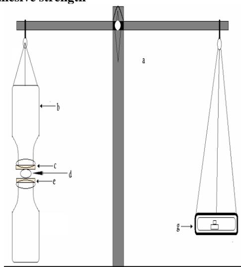
**Figure 2. Tablet adhesion retention period measurement apparatus**
